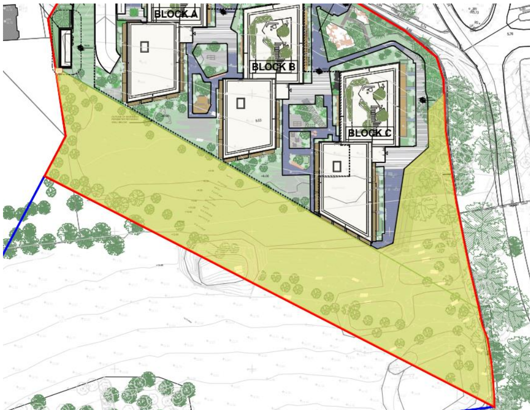
Figure 3.2 – Reprofiled area in yellow totalling 7400m 2
